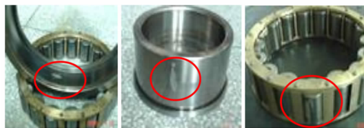
(a)轴承外圈故障 (b)轴承内圈故障 (c)轴承滚动故障
